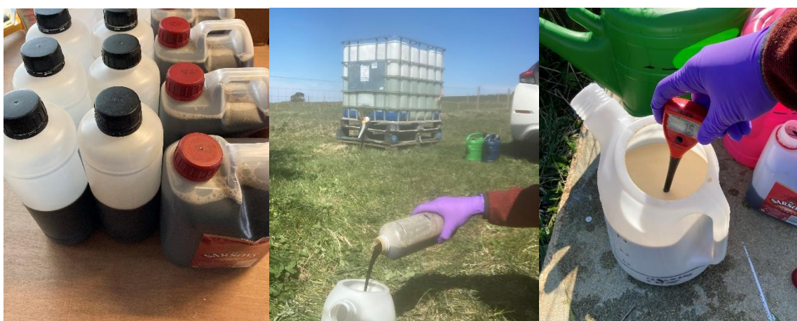
Figures 4a-c: “Organic” pH-balancing of homemade biodiesel co-product
